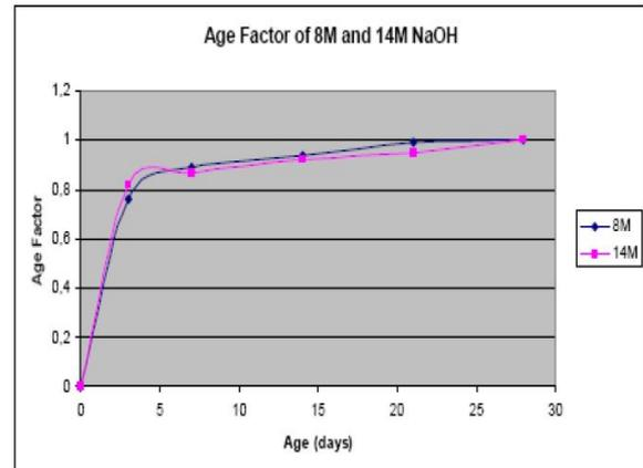
**Fig.4. Age factor of 8M and 14M NaOH based on the strength of Geopolymer concrete**
