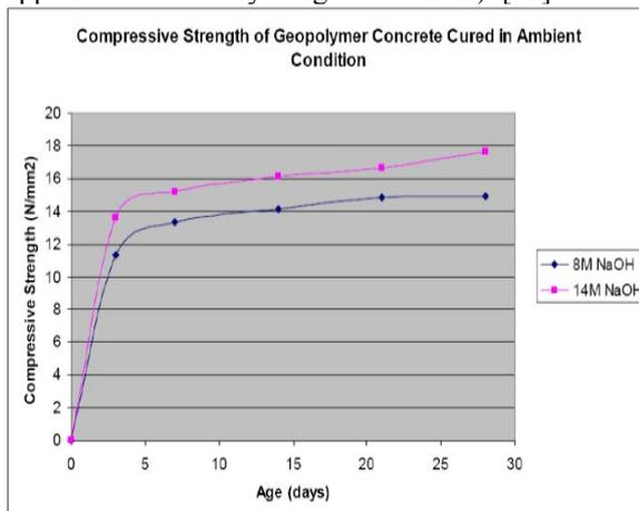
**Fig.3. Compressive Strength of GPC with different molarities of sodium hydroxide (NaOH)**
