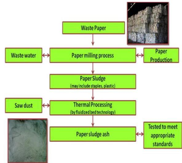
**Fig. 2.** Production process of WPMSA
